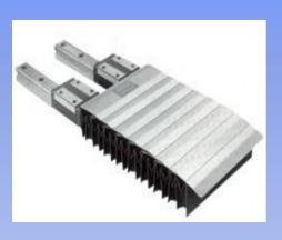
Metal Clad Bellow Covers are also available with over lapping of special .2 to.5 mm thk SS Sheet. Metal Sliding Flaps to protect its upper & side surface from direct fall of external influences. (Hot Chips). Metal Cladded (Metal Covered) Bellows are normally used where there is no space for compression of Bellows & where continuous machining process is going on.
