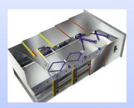
Telescopic Steel Covers are an important part of a machine tool to increase the runtime. The using of it makes possible perfect protection of the Guide-way, Balls-screw, etc. against mechanical influences like chips or chemical influences like coolants. Made from 1mm to 5mm thickness sheet of required material like SS,MS. Also provides good protection against accidents.
