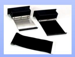
Rollway Covers are used when space is limited & other types of guide-way covers are not suitable for the protection of the machine ways & screws against damage from hot chips cutting oils, lubricants & abrasive partials. Construction consists of high tensile synthetic fabric or spring steel shade mounted on spring loaded, roller take up mechanism housed.
